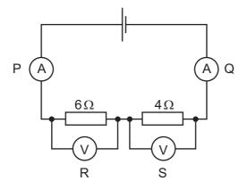
How do the readings on the meters in the circuit compare?
